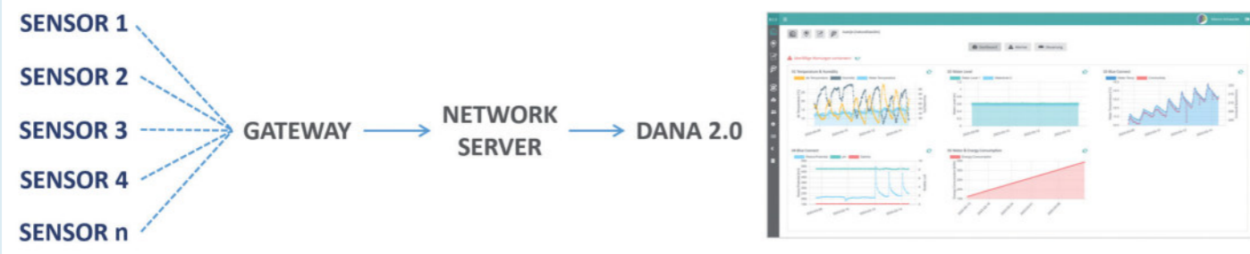
Figure 1: Functionality of data transmission via LoRa set
