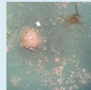
Figure 4: 14.06.2022: Foil not cleaned (NGF): Coatings of calcareous precipitates, brown crusts and green filamentous algae, occasionally also chironomid larvae (45x magnif.)
