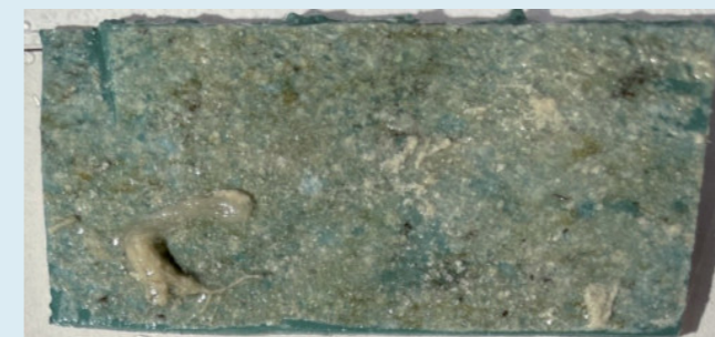
Figure 6: 13.09.2022: Foil not cleaned (NGF): left: Original view - right: magnifying glass view (approx. 45x magnif.). Coatings of calcareous precipitates, predominantly green coatings and bundles of dead, filamentous algae. - All images: KLS
