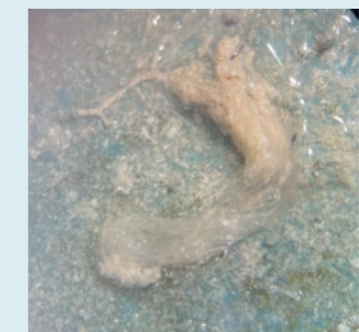
Figure 6: 13.09.2022: Foil not cleaned (NGF): left: Original view - right: magnifying glass view (approx. 45x magnif.). Coatings of calcareous precipitates, predominantly green coatings and bundles of dead, filamentous algae. - All images: KLS
